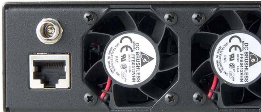
Picture 3: Far left side of RT-PoE3N rear panel
